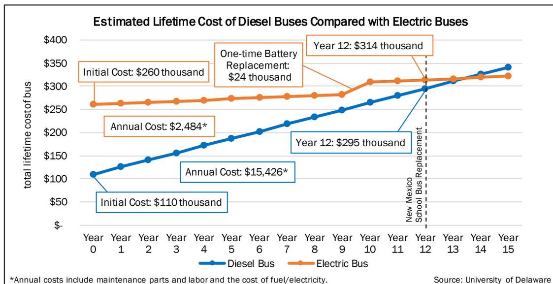
Electric school buses become more efficient and cost effective when used in a vehicle-to-grid (V2G) system. V2G systems are new systems designed to use the energy stored in the batteries of
