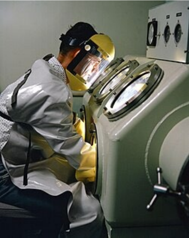
Image of a glovebox similar to those at LLNL which are too large for type B packaging
