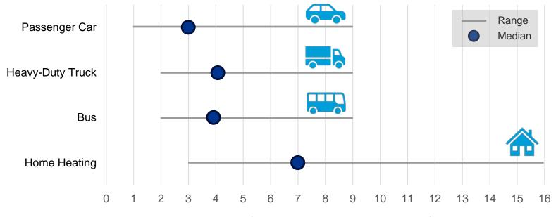
Energy Intensity of Hydrogen Relative to Direct Electrification
