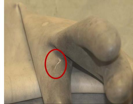
*Above, a glovebox glove that was breached at PF-4. Below, a rigging component that unexpectedly sheared under a load.*
