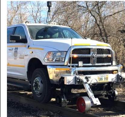
Machine Vision Track Inspection
