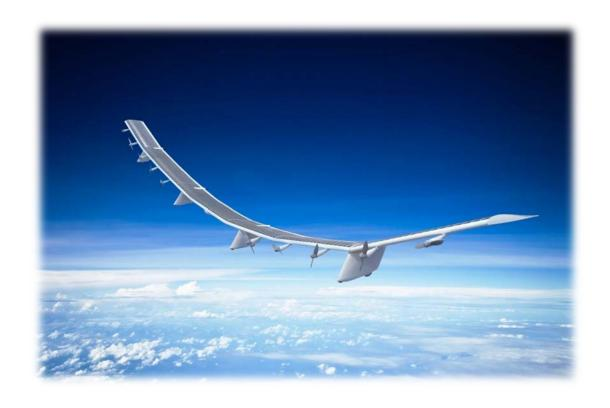
Unmanned solar-powered High Altitude Platform System
