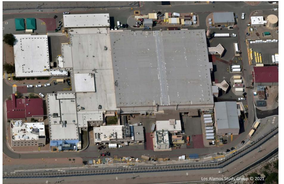
Seismic "demand" has increased x3 horizontally and x6 vertically since it was built (Keilers, NNSA, 2014).
