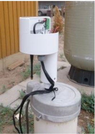
New acoustic groundwater monitoring devices, providing real time data (WellIntel)
