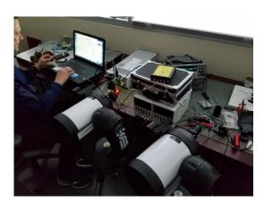
Prototype 1 – A 100m 10Gbps Single Channel Optical Wireless Simplex -Demo Delivered to Fortune 500 customer May 2017 for ~\$250,000 in Revenue
