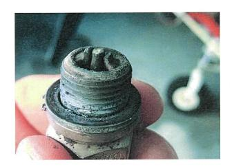
Lead is also a major safety issue, associated with aircraft engine failure -
