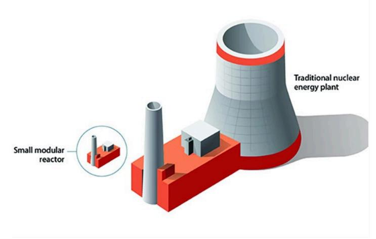
Small modular reactors are about 1/10 to 1/4 the size of a traditional nuclear energy plant due to compact, simplified designs. (Image credit: Idaho National Laboratory)
