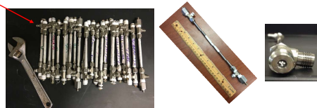
Membrane modules assembled for the DCMD experiments.
