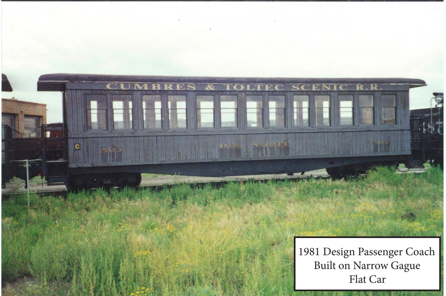
Earliest C&TS Passenger Cars Made of Modified Box Cars
