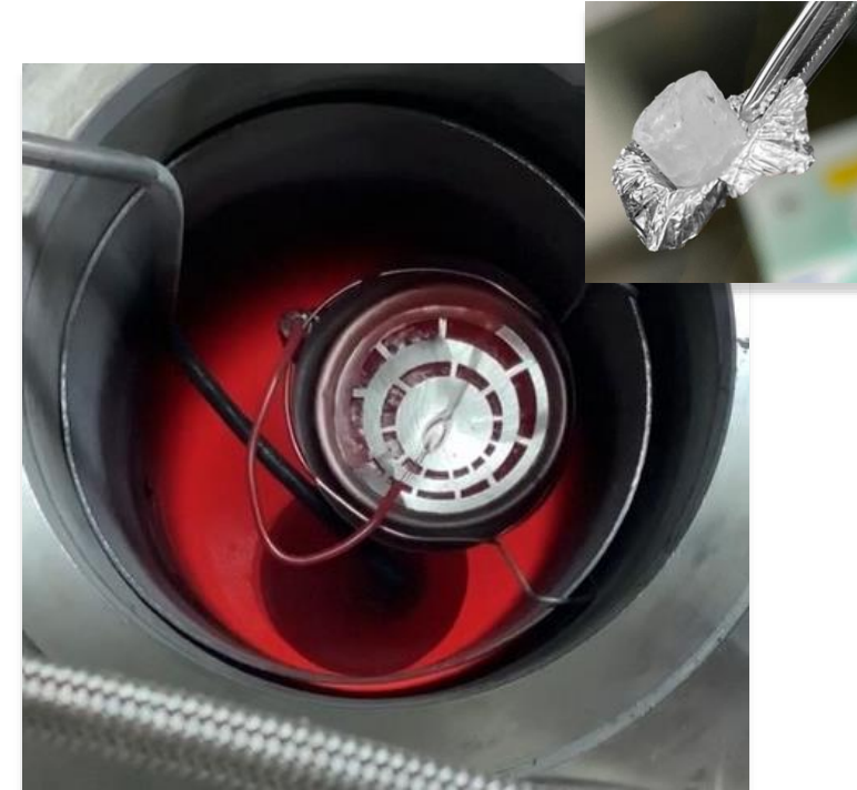
Liquid Fluoride Salt Coolant Flibe ( 2\text{LiF}-\text{BeF}_2 )
