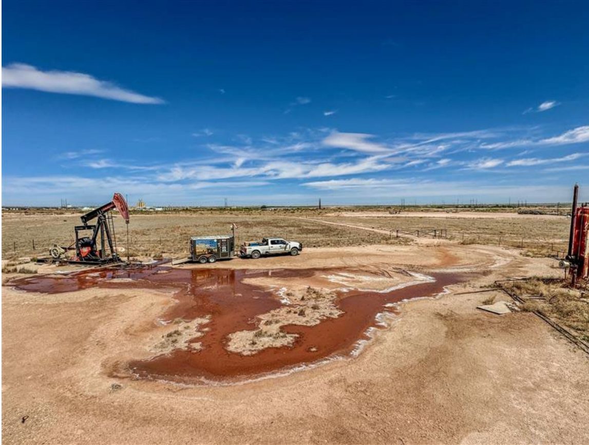
Pre plugging, produced water leak
