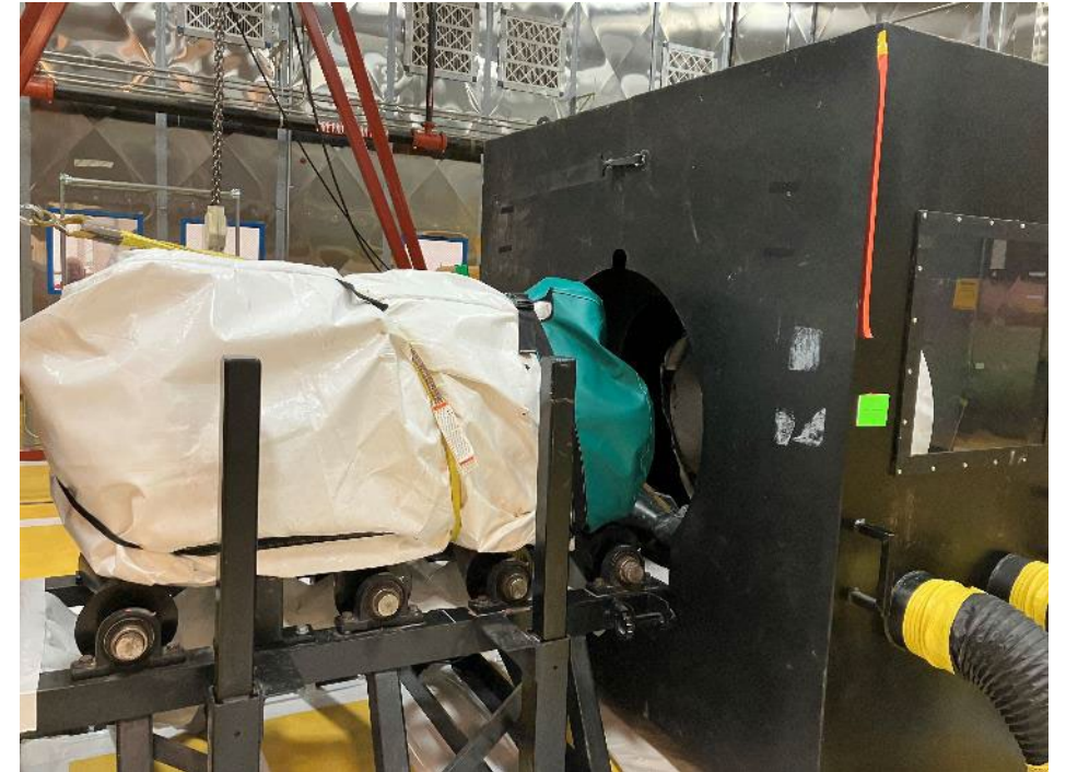
Practice Cut of Surrogate Corrugated Metal Pipe to Demonstrate Readiness
