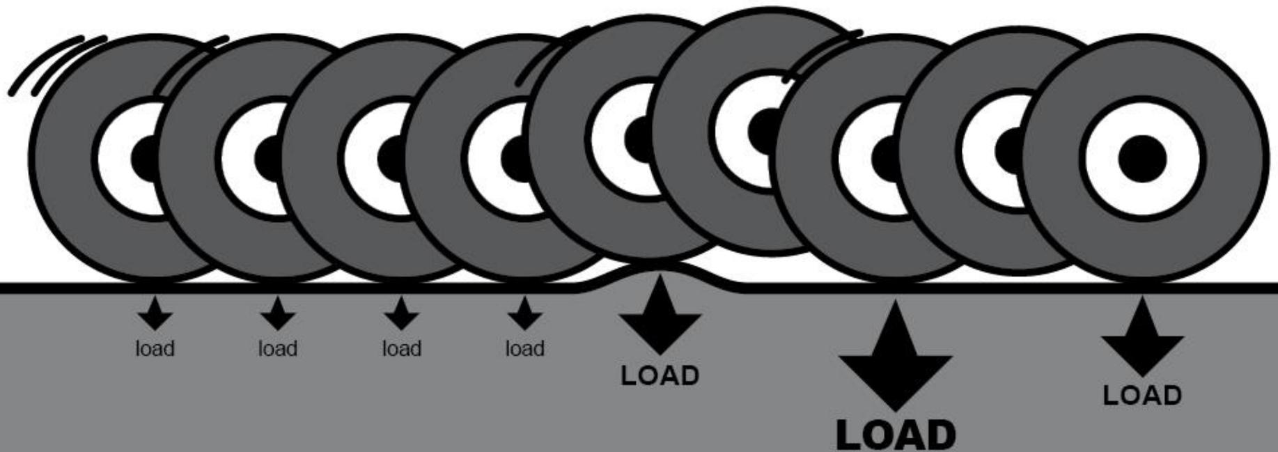
**Pavement roughness leads to higher dynamic loads on localized pavement sections, which increases pavement deterioration and fuel consumption as well as lowering ride quality. This also leads to a cycle of escalating deterioration rates with increasing roughness severity.**
