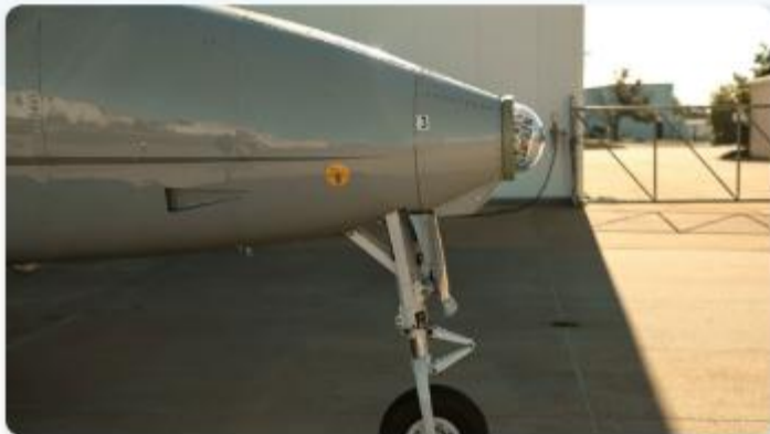
Boeing's Ultra Low-Cost Seeker sits mounted to a Beechcraft 1900 ahead of a captive carry test flight to evaluate baseline seeker target detection and tracking. (Photo by Chris Bishop)
