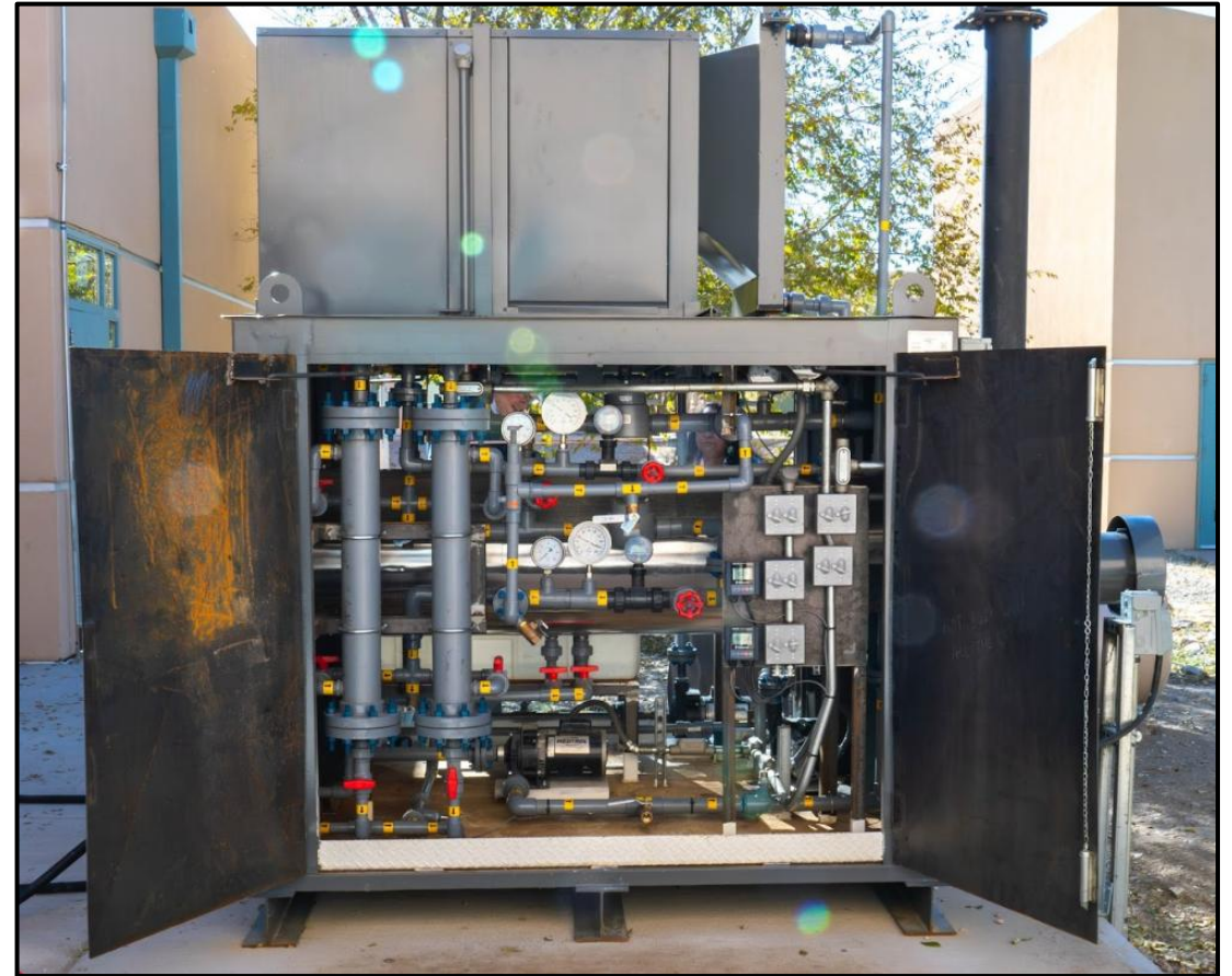
500 gallons per day, Pesco training unit NTU campus (Crownpoint, NM)
