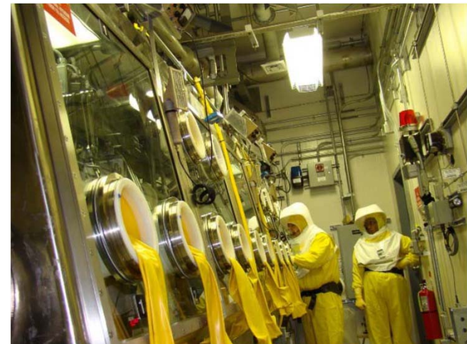
Glovebox Operations at Savannah River Site
