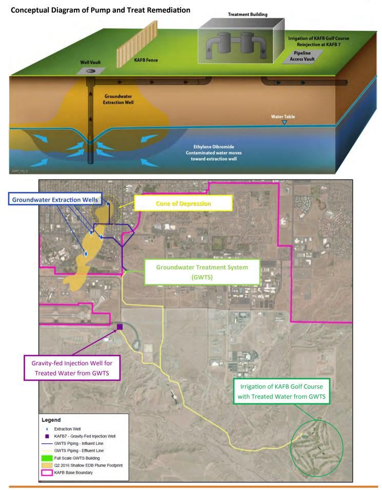
In March 2016, after three months of operating the first three groundwater extraction wells, a cone of depression was observed in the northern extent of the EDB plume. The cone of depression was the first milestone towards containment and collapse of the dissolved-phase EDB plume. The cone of depression appears to persist throughout 2016 even after groundwater extraction well KAFB-106233 is taken offline.
