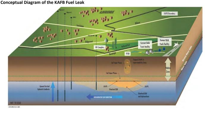
The conceptual diagram illustrates the nature and extent of fuel-related contamination across the site. Fuel originally floated on the water table but has, over time, become submerged as regional groundwater levels rise. The LNAPL migration path through the subsurface was influenced by the local geology, the properties of the compound and soil, and the height of the water table over time. This conceptual site model continues to be evaluated as data is collected and data gaps are closed.
