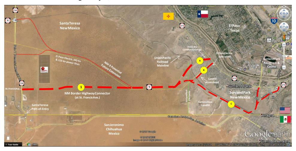
The NM Border Highway Connector has three potential alternative routes (A,B,C) within the city limits of Sunland Park
