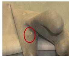
Above, a glovebox glove that was breached at PF-4. Below, a rigging component that unexpectedly sheared under a load.
