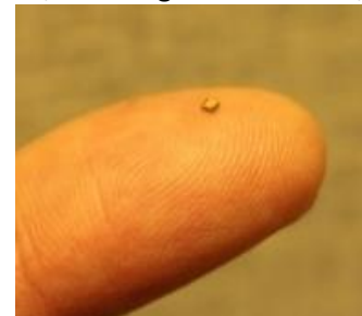
Figure 1. Laser array chip forms an optical wireless link at 10Gbps which projects an invisible eye safe light field the size of a house stabilizing an optical mesh network
