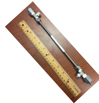
Membrane modules assembled for the DCMD experiments.
