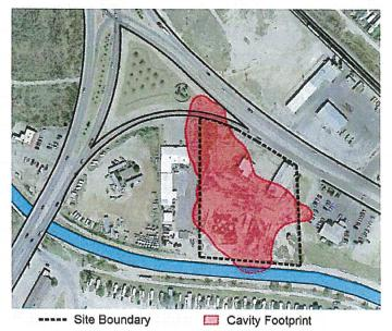
damage to infrastructure and property, disrupt interstate travel, commerce, and local agriculture, and pose a threat to public safety. The Carlsbad Brine Well Remediation project aims to design and implement a plan to minimize these impacts by filling the subsurface cavity with grout to stabilize the existing underground void created by operation of the I&W facility.
