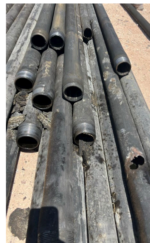
Figure 8. Corroded Production Tubing
