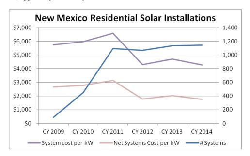
This effect can be explained somewhat in that installation labor cost has leveled out at about \$5,500 per installation, while the module cost per installation has fallen (as shown in the following chart). Thus, labor costs as a percentage of total cost has increased almost in inverse ratio to the drop of module costs.
