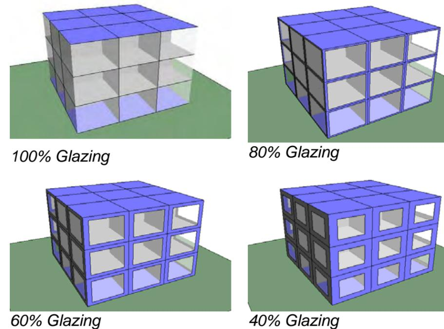
Figure 3-4 Glazing-to-Wall Ratio
