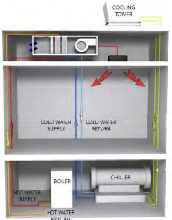
Figure 3-17: Four-Pipe Fan Coil System
