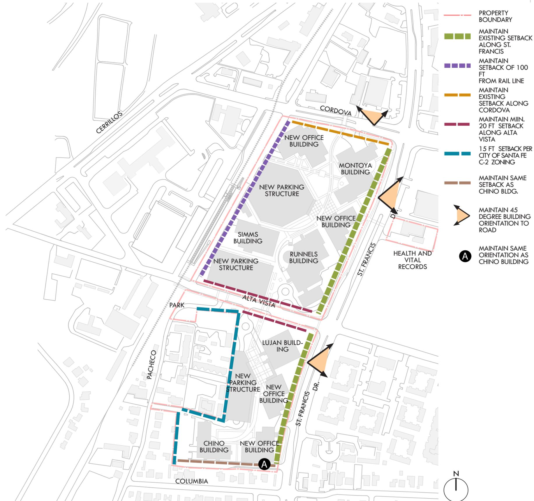
Figure 4-3: Setback & Orientation Concept Diagram
