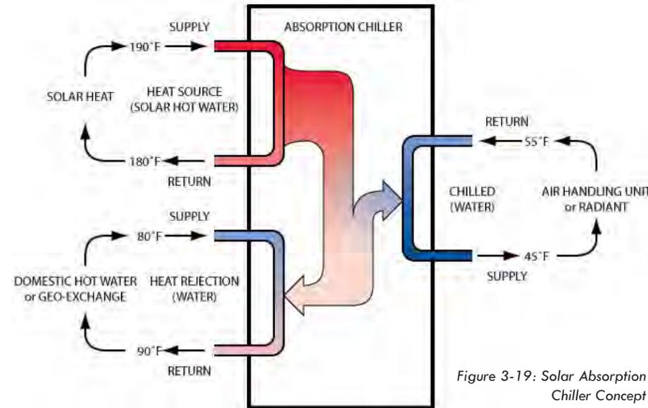
Figure 3-19: Solar Absorption Chiller Concept
