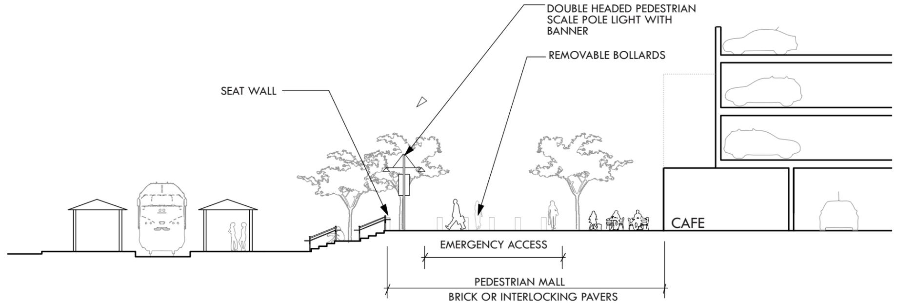
Figure 4-13: Transit Mall - Cross Section
