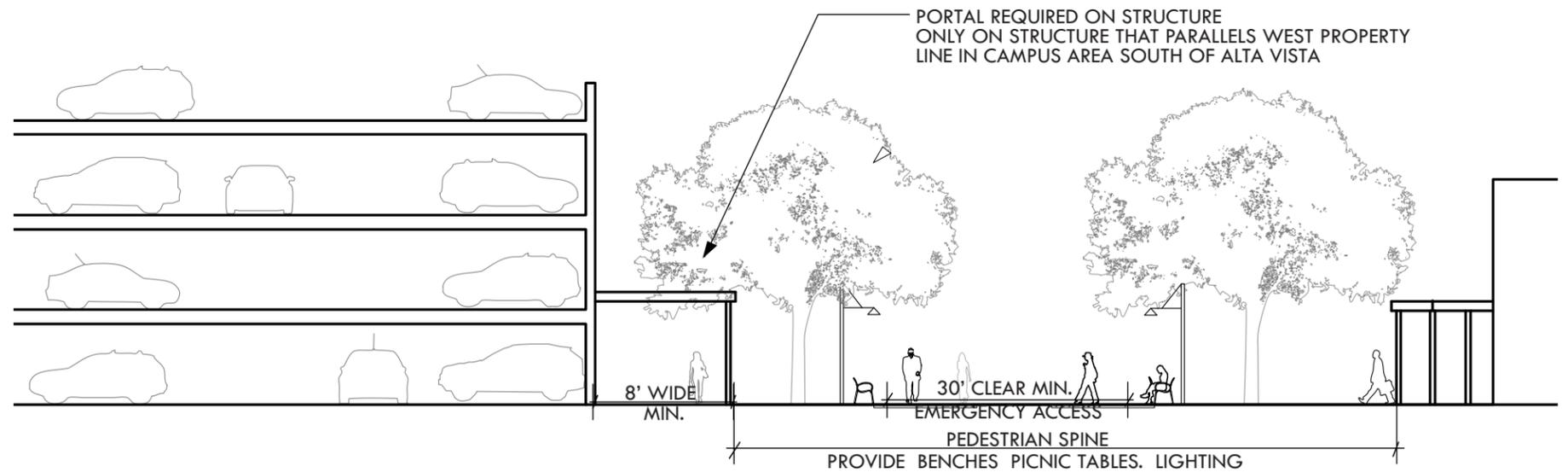
Figure 4-14: Campus Pedestrian Spine - Cross Section near Manuel Lujan Building
