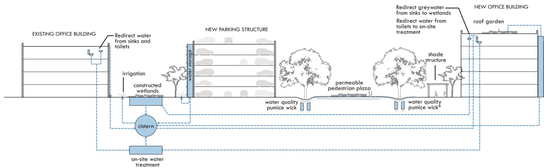
Figure 2-15: Water Harvesting Conceptual Diagram
