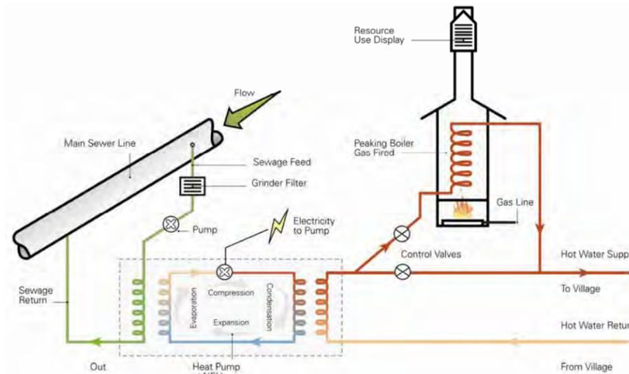
Figure 3-14: Example of Sewer Heat Recovery
