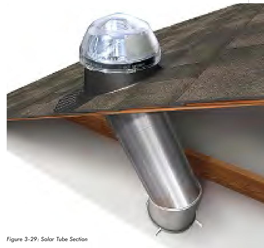
Figure 3-29: Solar Tube Section
