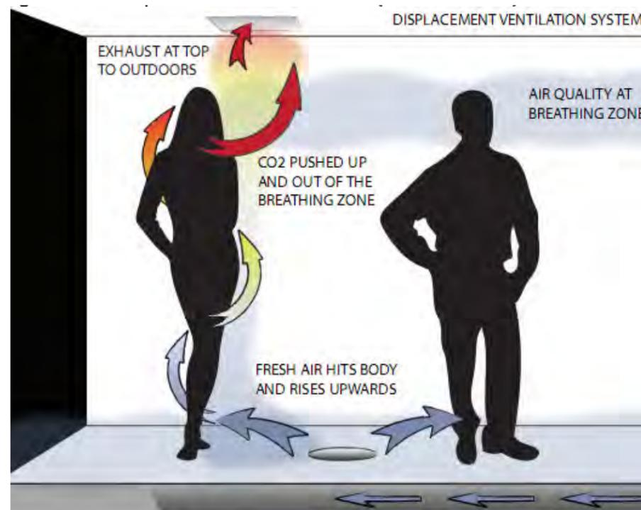
Figure 3-22: Displacement Ventilation
