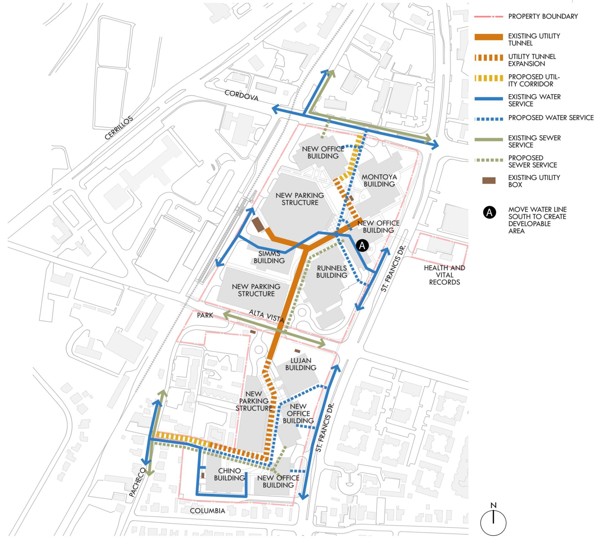
Figure 4-6: Utility Concept Diagram
