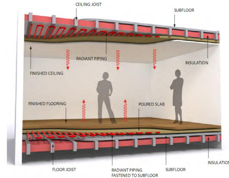
Figure 3-18: Radiant Heating and Cooling
