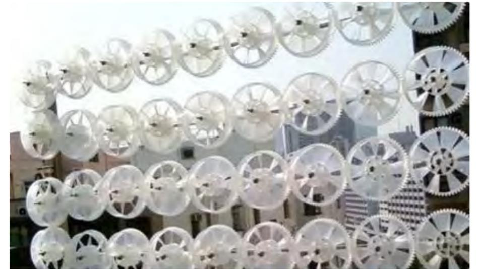
Figure 3-11: Micro-Wind Generators
