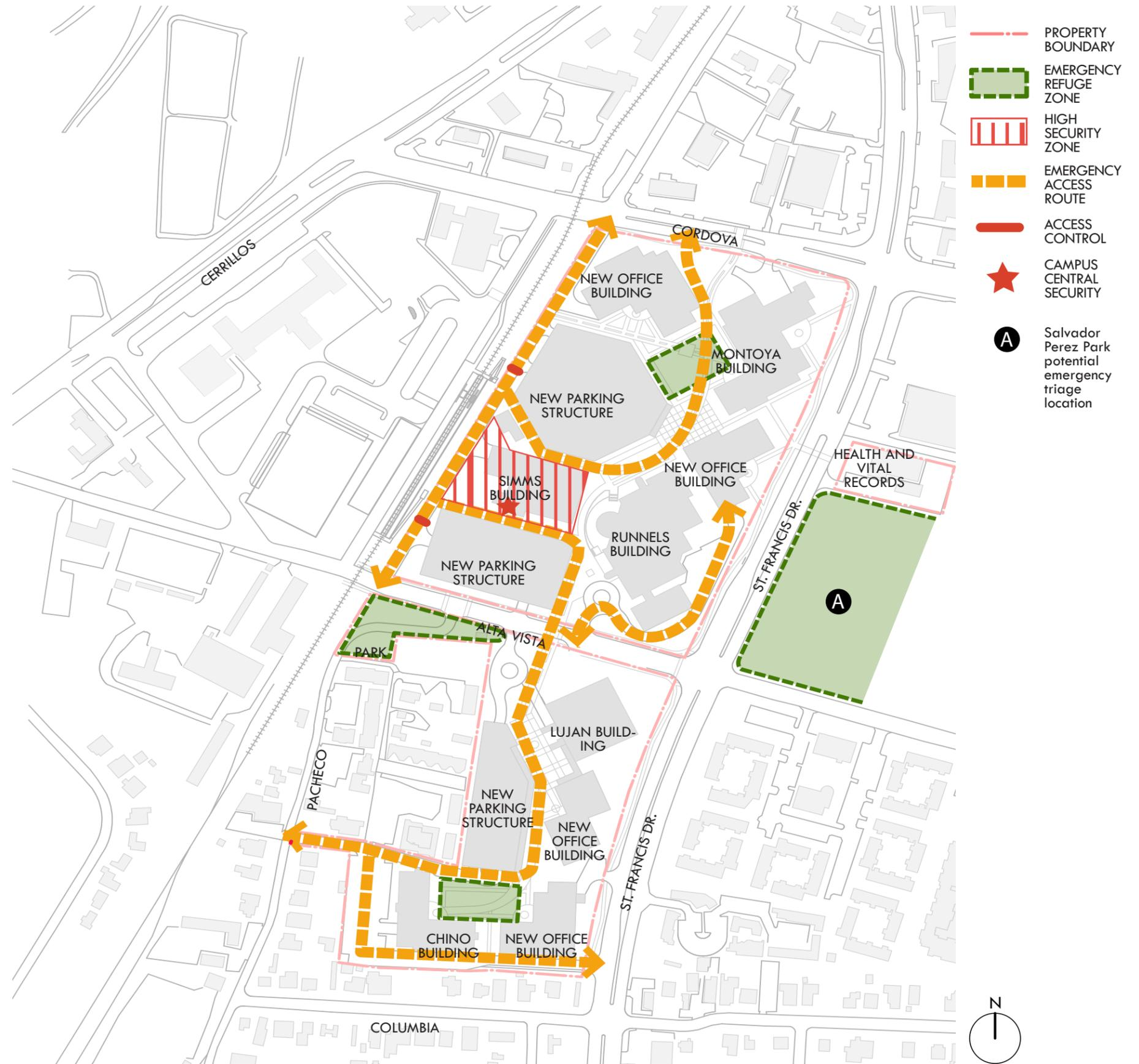
Figure 4-9: Security Concept Diagram
