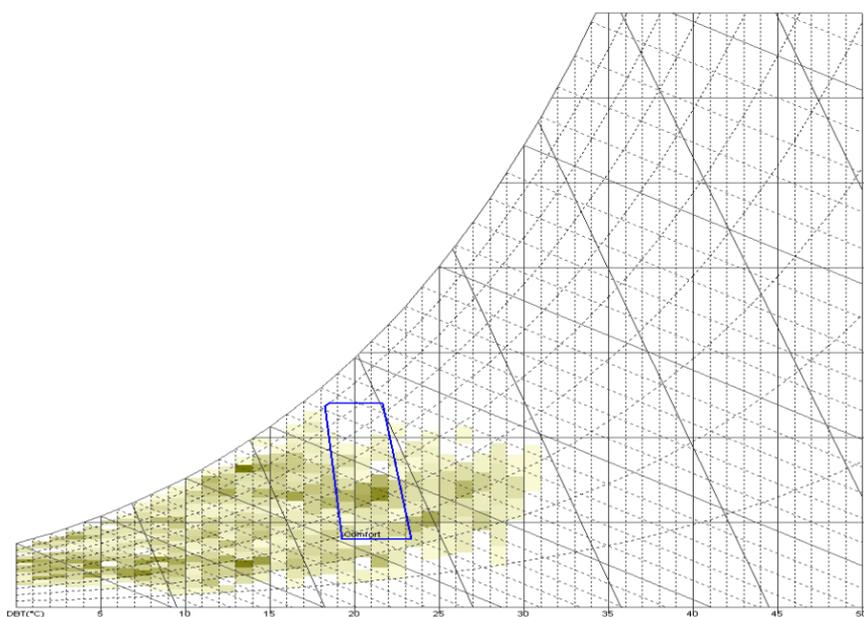
Figure A-61: Psychrometric Chart Showing Relative Frequency of Outdoor Air Conditions in relation to ASHRAE Comfort Zone (Fall)
