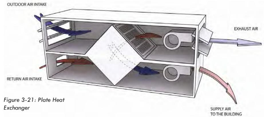
Figure 3-21: Plate Heat Exchanger
