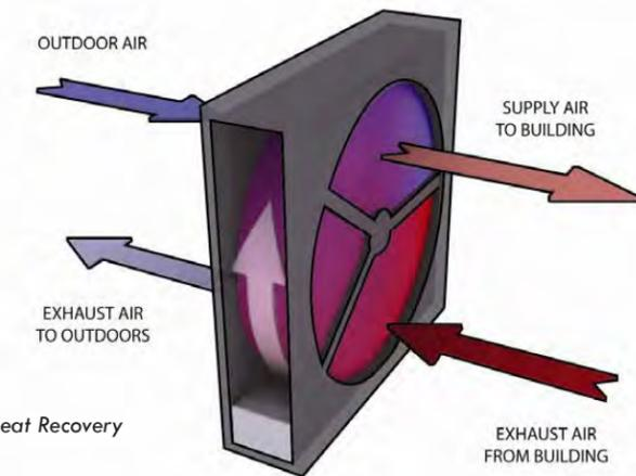
Figure 3-21: Heat Recovery Wheel
