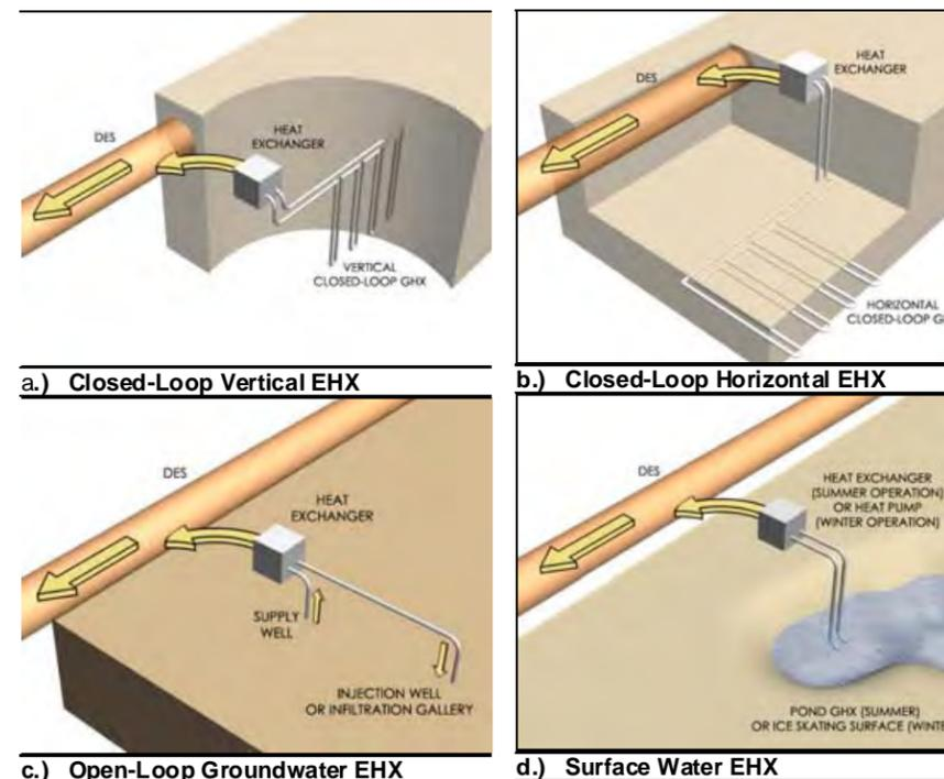
Figure 3-12: Earth Source Exchange Systems
