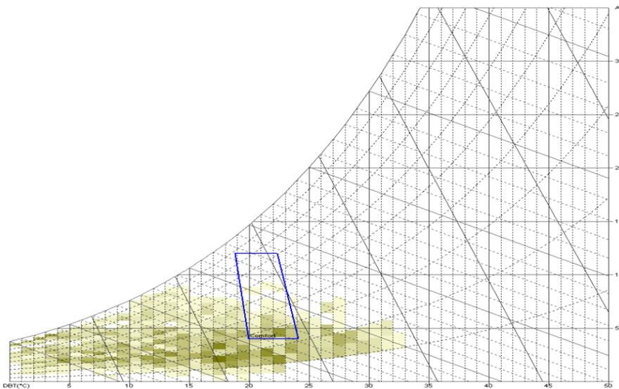
Figure A-59: Psychrometric Chart Showing Relative Frequency of Outdoor Air Conditions in Relation to ASHRAE Comfort Zone (Spring)
