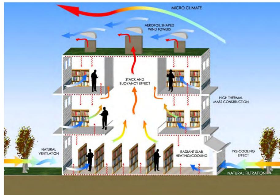
Figure 3-9: Example of Natural Ventilation with an Atrium (Potential for Runnels and Montoya Buildings)
