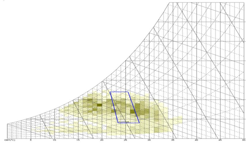
Figure 60: Psychrometric Chart Showing Relative Frequency of Outdoor Air Conditions in Relation to ASHRAE Comfort Zone (Summer)
