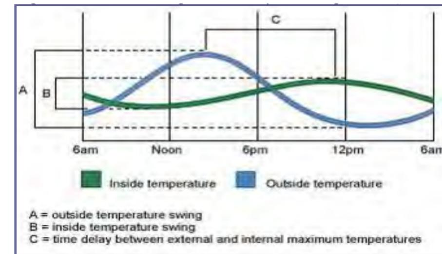
Figure 3-3 Thermal Lag of a Heavy Building Mass
