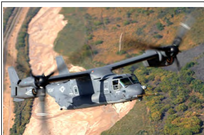
The CV-22 has rotating engines to operate as a turboprop aircraft in flight and a helicopter when landing or taking off. During training in the proposed low altitude training area, the CV-22 would operate as an aircraft.
