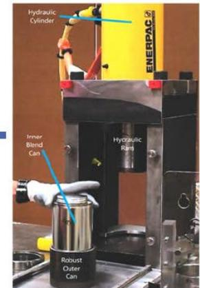
Lids are press-fit to close Robust Outer Container (ROC)
