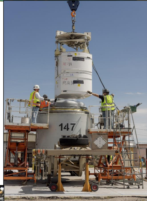
Crews use a mobile-loading unit to place containers of LANL's legacy transuranic waste into casks for transport to WIPP
