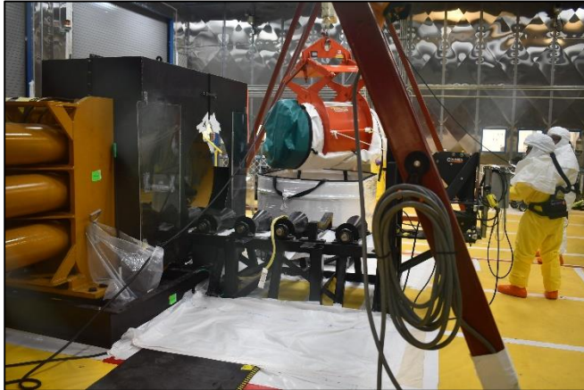
N3B Waste Retrieval Operations crew guide a cut section of corrugated metal pipe (CMP) filled with cemented transuranic waste into a standard waste box.
