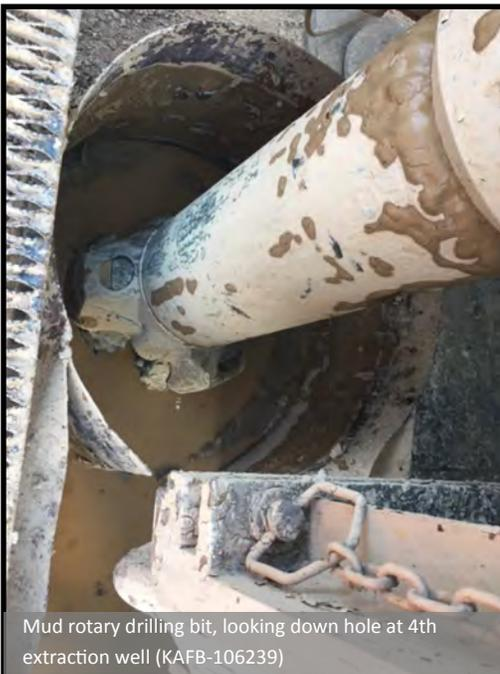
Mud rotary drilling bit, looking down hole at 4th extraction well (KAFB-106239)
