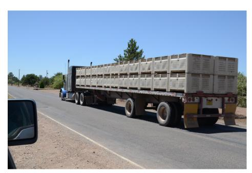
Pictured at left is a semi hauling an onion load estimated to be at least 90,000 pounds. It is traveling on Solana Road, which is plagued with potholes, shoulder issues and a rating of 60,000 pounds.
