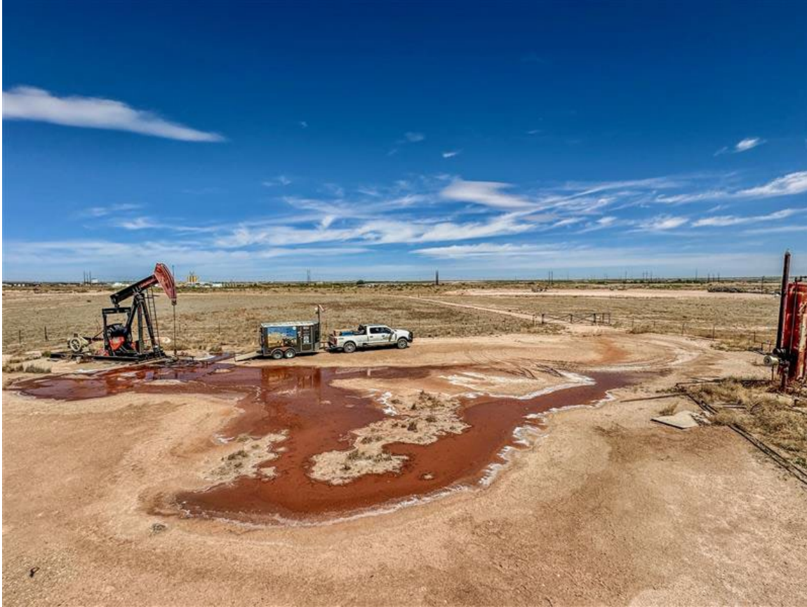
Pre plugging, produced water leak
