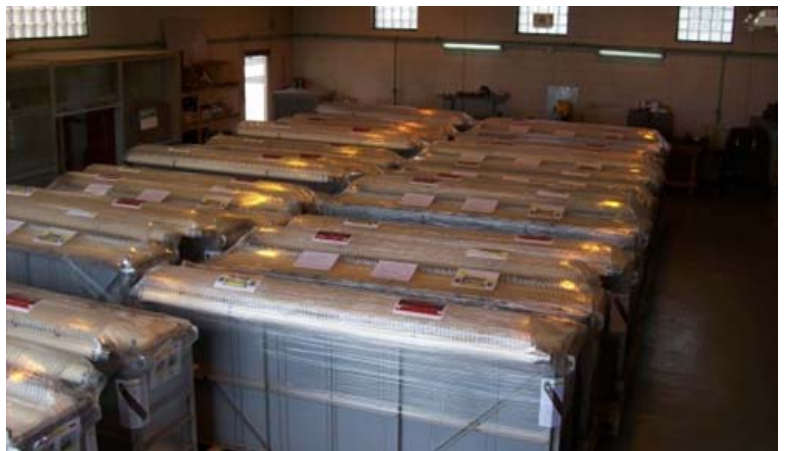
Village of Los Lunas new MBR cassettes prior to installation Funded by CO SAP
