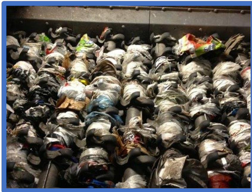
Figure 3. Plastic bags get tangled in sorting systems at materials recovery facilities (MRFs) and require the sorting system to shut down to clean the material from the gears.
